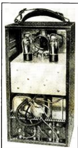
The rear view shows how compactly the batteries fit the cabinet. Below, Fig. 1.
